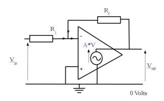
$$G = \frac{V_{\text{out}}}{V_{\text{in}}} = \frac{-R_f A}{[R_r(A+1) + R_f]}$$
