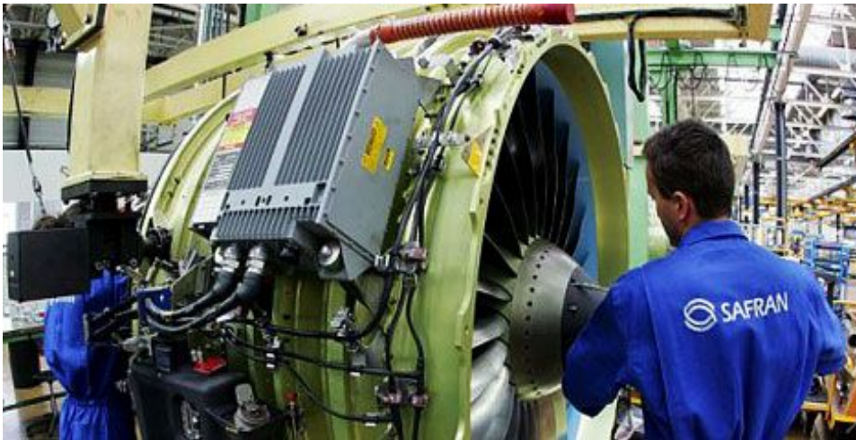
Jet engine control circuits, which decide how/when fuel is injected - 5V/50 mA
