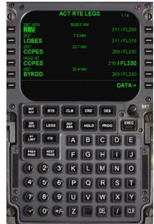
Flight management system from Boeing 737.
