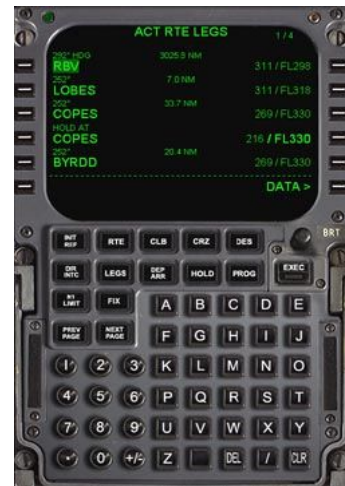
Figure 1: An example of a display on an embed system. It may not have fancy graphics but this display to a modern computer controlling a Boeing 737's flight path.
